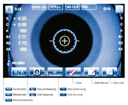
Intuitive icons provide the user an easier operating circumstances, and make the measurement become more convenient and the data to be measured more accurate and fast
